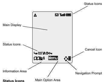
The status icons are displayed according to the currently activated functions. The Antenna, Signal and Battery icons are always displayed when the handset is switched on and connected to a network.
